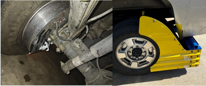
Brake-Wear and Tire-Wear On-road measurements for heavy- and light-duty vehicles
