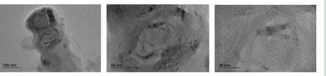
Presence of sub-micrometric objects in the particulate samples that also displayed Raman spectra very close to those of reference CNTs (likely actually present in these particulate samples).
