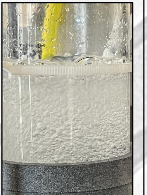
Without the necessity to renew the salt solution, the generated particle concentration and size distribution remains constant, as the consumption of the salt solution is very low.
