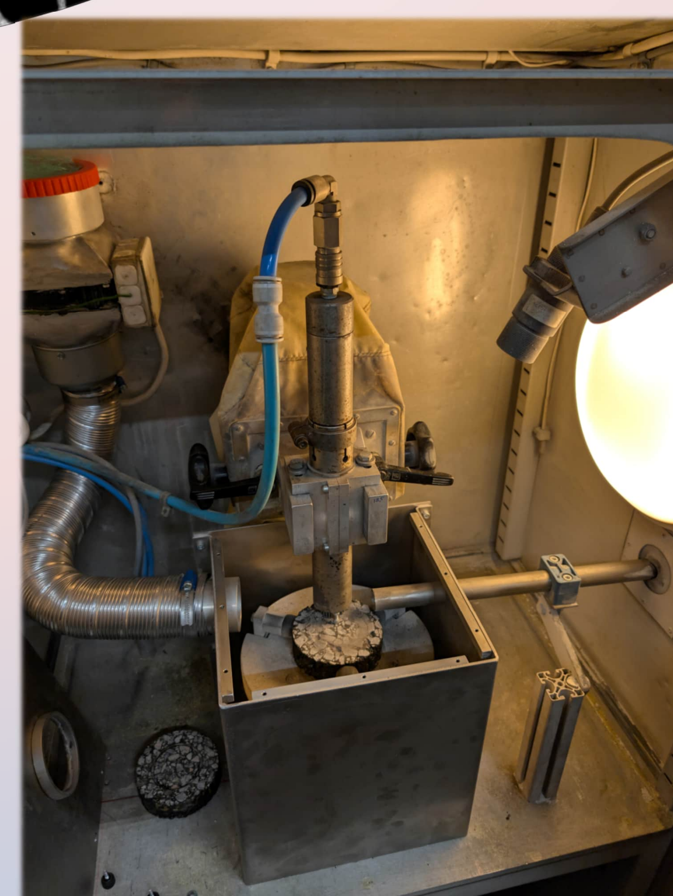
Figure 5. Tröger Road Wear screening method at VTI (Linköping, Sweden).
