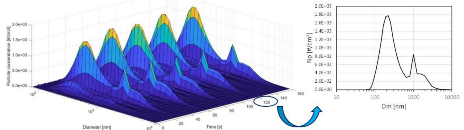
A significant fraction of the particles falls in the 90 - 650 nm size range while particles larger than 800 nm gives a smaller contribution. The different sizes of the particles suggest they originate from different formation mechanisms: the high disc temperature is responsible for the emission of smaller size particles; the larger particles are generated by the mechanical abrasion.
