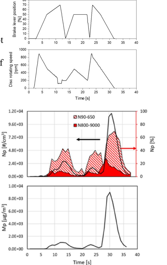
BWPs range between 90 nm and 0.4  $\mu$ m. The time series data for number concentration exhibits a two-peak pattern, at 200 and 1000 nm, during each braking event.
