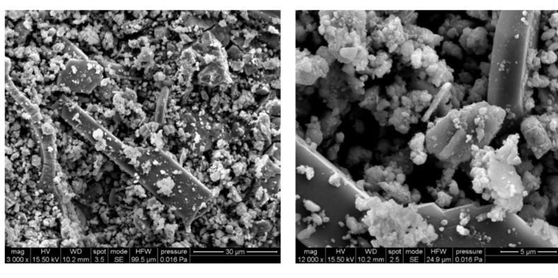
The presence of both smooth and fractured surfaces implies different wear and transformation mechanisms, such as thermal degradation, adhesion, and abrasion.
