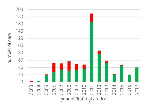
Distribution of the filter failure rate as a function of vehicle operating time (green: <250,000 cm<sup>-3</sup> red: > 250,000 cm<sup>-3</sup>)
