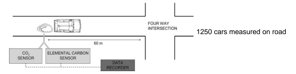
**Beaton et al., 1995:** The emission distribution is highly skewed; the half of the fleet with the lowest emissions contributed less than 10% of the CO and HC, while a few high-emission vehicles dominated the mean values. In this instance, 7% of the vehicles accounted for '50% of the on-road CO emissions, and 10% of the vehicles accounted for 50% of the on-road HC emissions.
