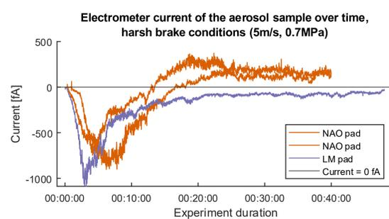
Figure 2: Aerosol current over time.
