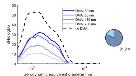
Figure 4: Aerodynamic particle size distribution of negatively charged particles (LM, mild conditions) selected with the DMA (no BPC). The mean APS size distribution for the same material and condition is shown for comparison (black, dashed line), and the percentage of particles detected with an APS (dark blue) compared to a CPC is shown in the pie chart show.
