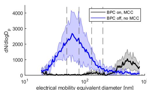
Figure 3: SMPS size distribution of negatively charged particles (LM, mild conditions) with the bipolar charger turned on and off. Vertical lines indicate the particle diameters: 50, 80, 130 and 200 nm.
