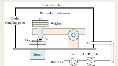
Figure 1: Pin-on-disc tribometer
