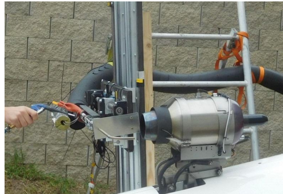
Cooling of the sample probe at high load
