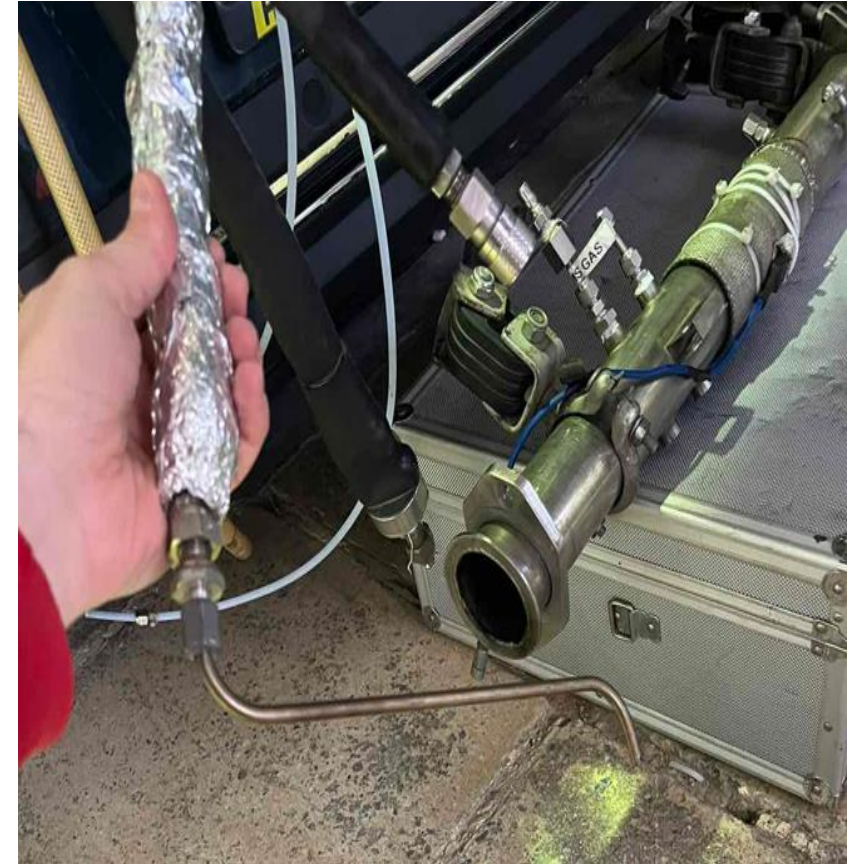
Exhaust pipe and heated line
