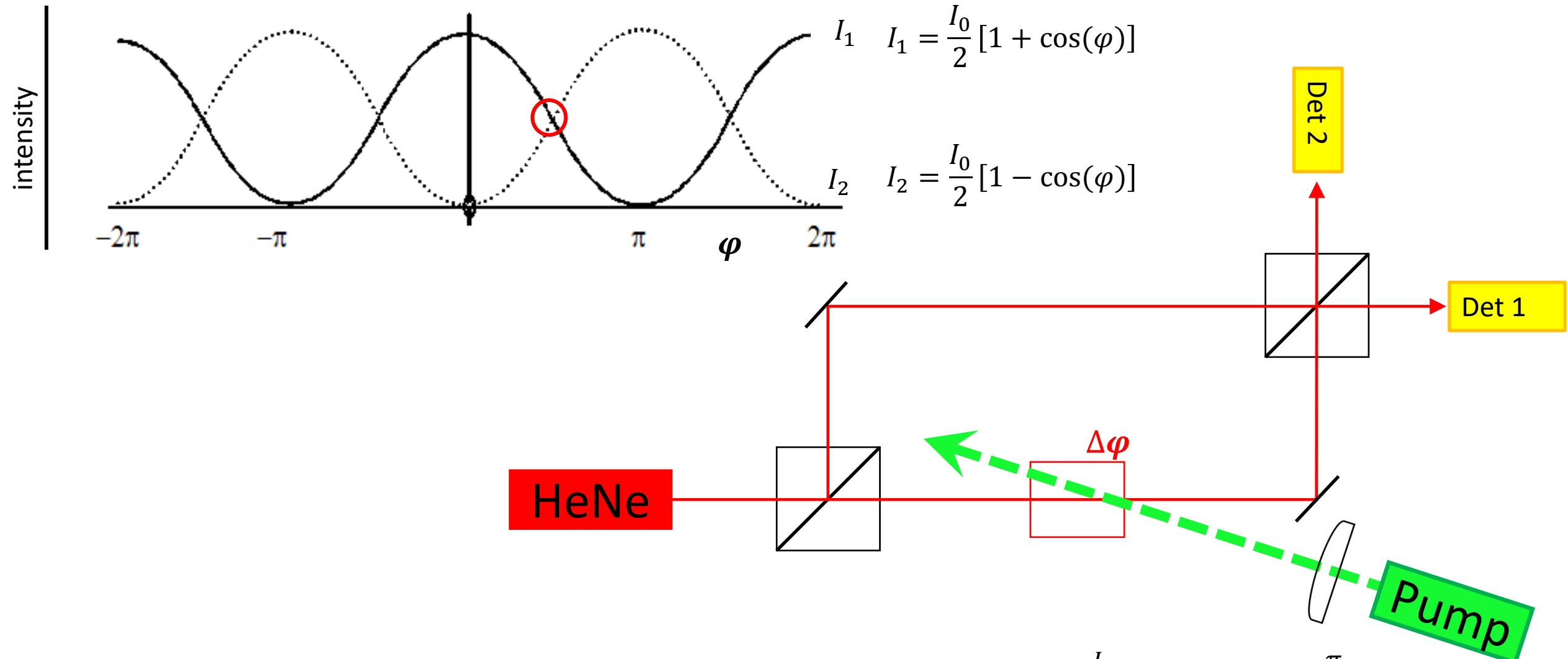
Highest **sensitivity** in  $\varphi$  change – the interferometer in **quadrature** ( $I_1 = I_2 = \frac{I_0}{2}$ ), e.g. at  $\varphi_o = \frac{\pi}{2}$ .
