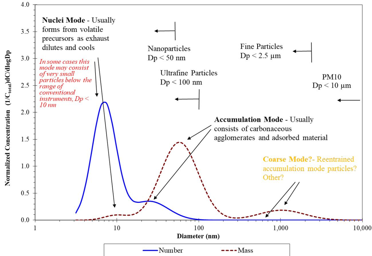
Gas turbine size distribution with certification sampling system,
