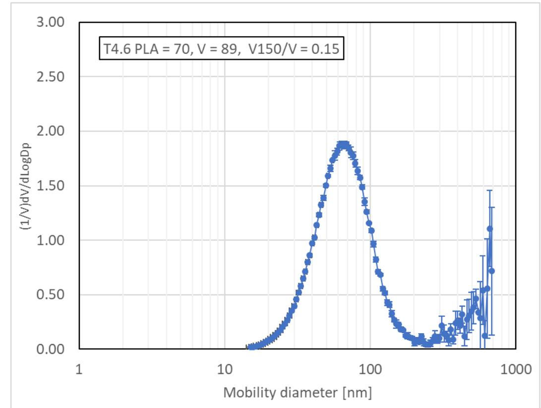
SMPS operated in low flow mode 0.3 Lpm/3 lpm – sizing range 15 to 690 nm
