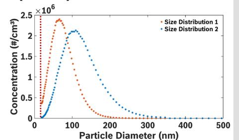
Comparison of measured LII signal peaks with SMPS data suggests the possibility of **particle sizing**.
