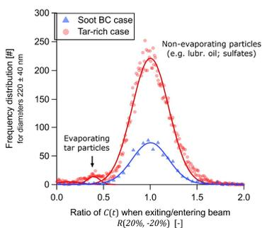
Figure 2. Identification of evaporating but non-incandescing tar particles. The frequency distributions are highlighted by Gaussian fits, representing random error. Evaporating particles only occurred in the tar-rich case.
