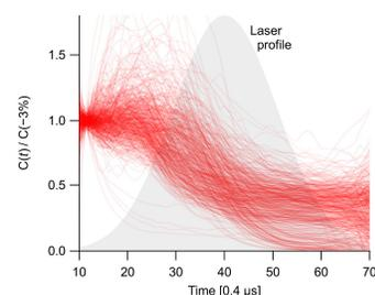
Figure 3. Evaporation trends of tar particles. Each red line corresponds to the lowest panel of Figure 1d. Each curve has been normalized to  $C(-3\%)$ , which is normally used for coating-thickness analysis [2,3].
