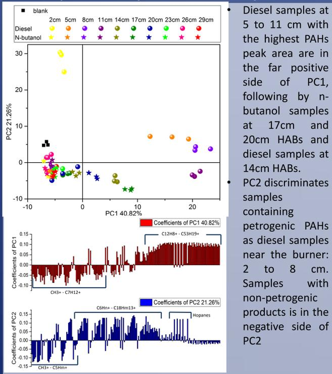
Diesel samples at 5 to 11 cm with the highest PAHs peak area are in the far positive side of PC1, following by *n*-butanol samples at 17 cm and 20 cm HABs and diesel samples at 14 cm HABs. PC2 discriminates samples containing petrogenic PAHs as diesel samples near the burner: 2 to 8 cm. Samples with non-petrogenic products is in the negative side of PC2
