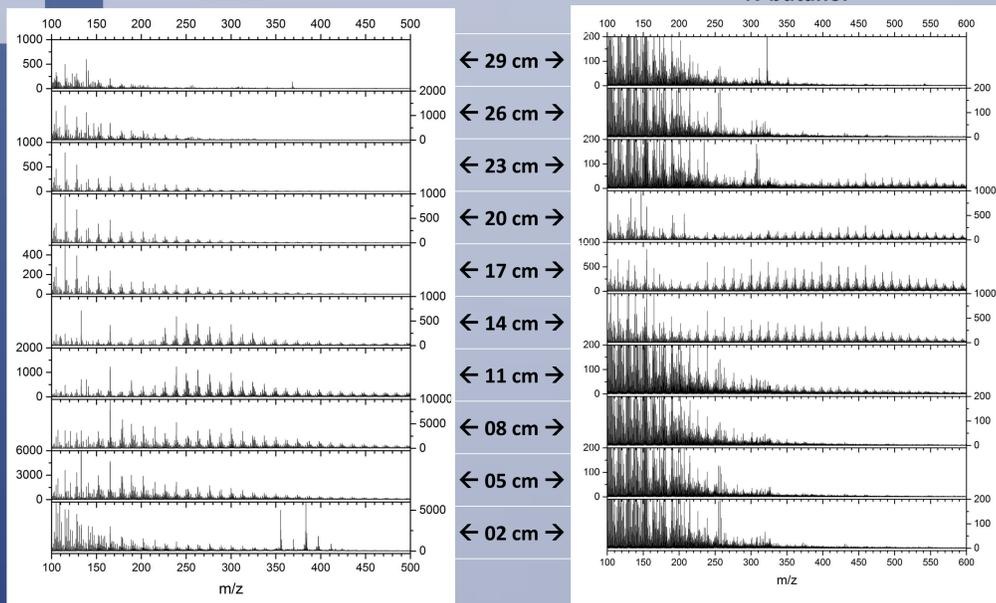
SIMS mass spectra of samples from diesel flame and *n*-butanol flame.
