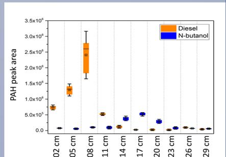
Box plot of PAHs integrated peak area from SIMS mass spectra of diesel samples and *n*-butanol samples.
