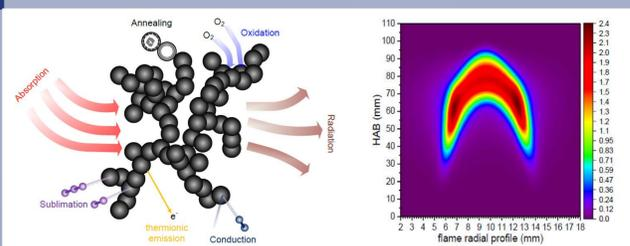
Soot aggregate illustrating the process influencing the collection of the LII signal and an example of LII signal from methane flame [4]
