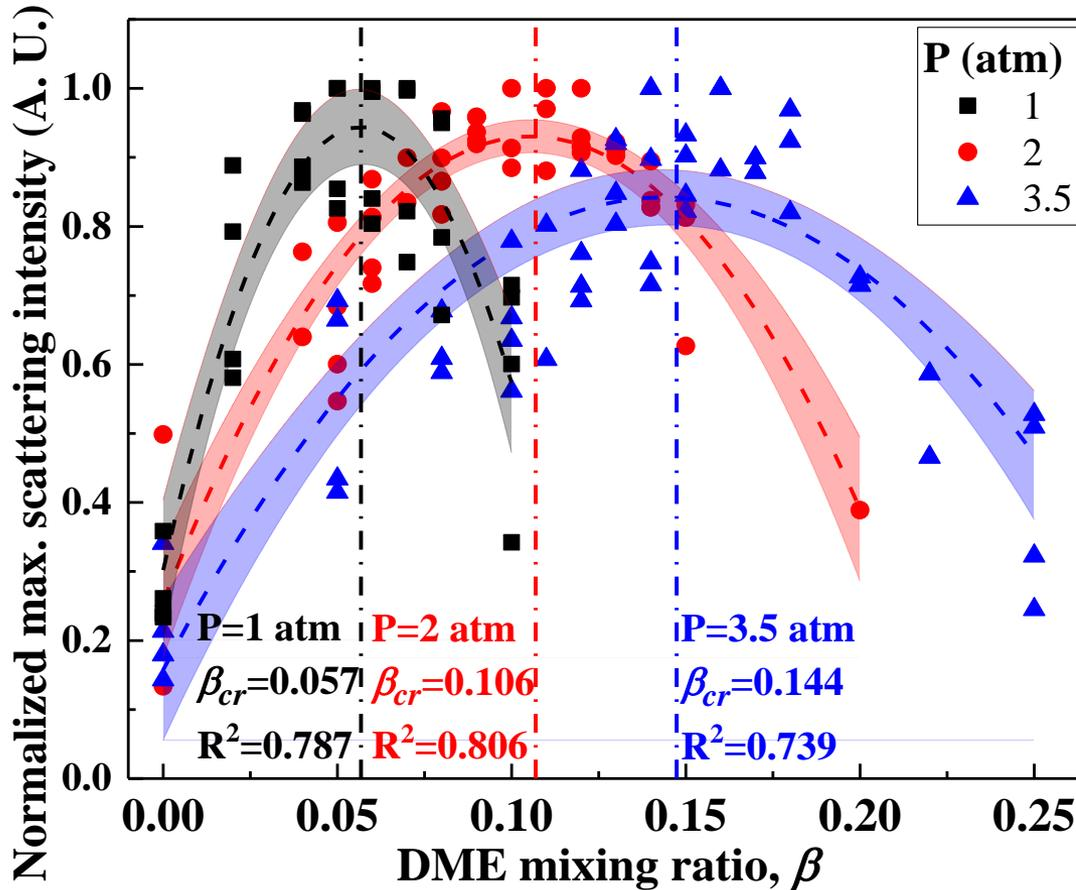
The range of  $\beta$  in increasing soot propensity expands with pressure.
