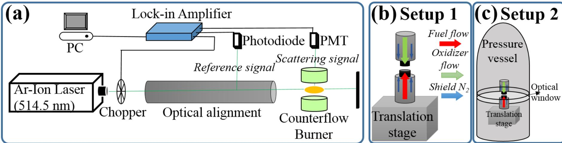
Schematics of experimental apparatus: Light scattering setup (a), and atmospheric counterflow burner (b)
