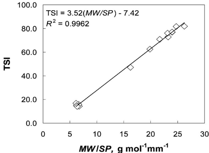
Fig. 3. Relationship between TSI and MW/SP ratio for prototype JP-900 fuel mixtures.
