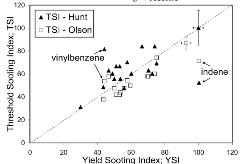
Fig. 6. Two sets of literature TSIs [9,27] plotted versus the measured YSIs. For clarity, error bars are shown for only one data point in each set; they represent the  $\pm 3\%$  total uncertainty in YSI, the  $\pm 15\%$  precision of TSI-Hunt, and the  $\pm 7\%$  precision of TSI-Olson.
