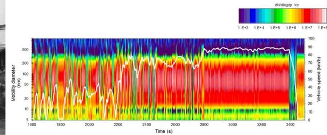
Fig 2: Vehicle Speed and particle size distribution as a function of time, from [3]
