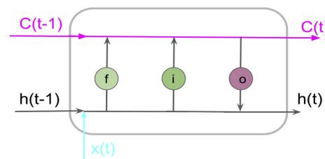
Fig 4: Schema of an LSTM,  $x(t)$  represent the input at time  $t$ ,  $h(t-1)$  the prediction at time  $t-1$ ,  $h(t)$  the prediction at time  $t$ ,  $f$  the forget gate at time  $t$ ,  $i$  the input gate at time  $t$ ,  $o$  the output gate at time  $t$  and  $C(t)$  the cell state at time  $t$ . Adapted from [8].
