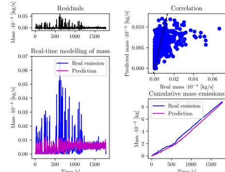
Fig. 7: Soot mass estimation from GMD, GSD and PN using the FA-method
