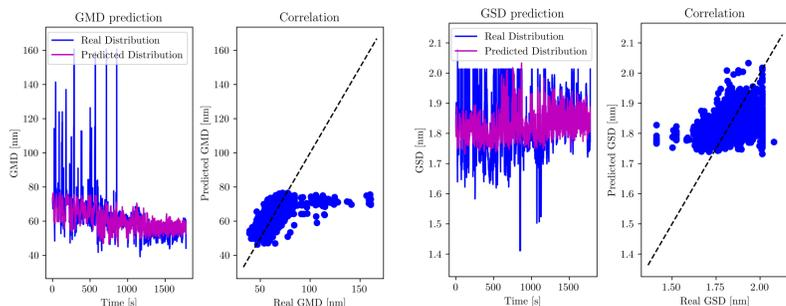
Fig. 6: PN, GMD and GSD prediction using an LSTM model
