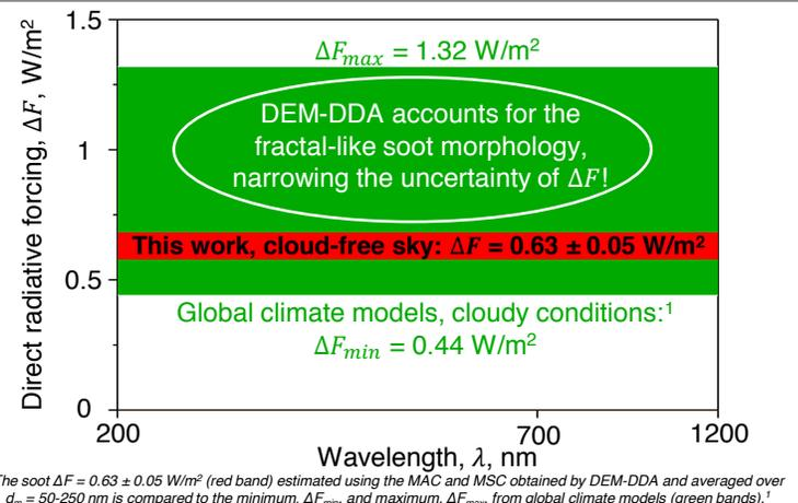
The soot  $\Delta F = 0.63 \pm 0.05 \text{ W/m}^2$  (red band) estimated using the *MAC* and *MSC* obtained by DEM-DDA and averaged over  $d_m = 50\text{-}250 \text{ nm}$  is compared to the minimum,  $\Delta F_{min}$ , and maximum,  $\Delta F_{max}$ , from global climate models (green bands).<sup>1</sup>
