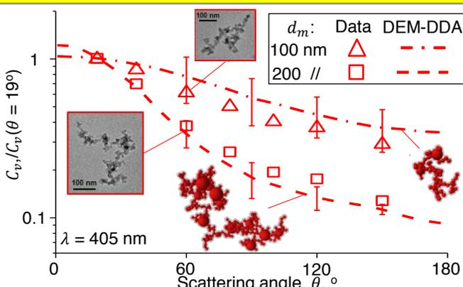
Differential scattering cross-section,  $C_v$ , of soot agglomerates with mobility diameter,  $d_m = 100$  (dot-dashed line, triangles) and 200 nm (broken line, squares) estimated by DEM-DDA (lines) or measured in premixed flames (symbols) and normalized with respect to scattering angle,  $\theta = 19^\circ$  at wavelength,  $\lambda = 405 \text{ nm}$ .
