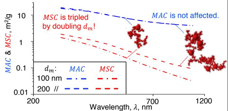
Mass Absorption, *MAC*, and Scattering Cross-sections, *MSC* of DEM-derived mature soot agglomerates with  $d_m = 100$  (dot-dashed lines) and 200 nm (broken lines) estimated by DDA as function of  $\lambda$ .
