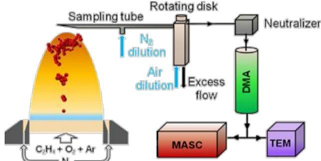
Soot agglomerates are sampled and diluted above a premixed ethylene flame with equivalence ratio of 2.1. The diluted sample is directed to a differential mobility analyzer (DMA) and then to a multiple angle scattering chamber (MASC) or collected for transmission electron microscopy (TEM).
