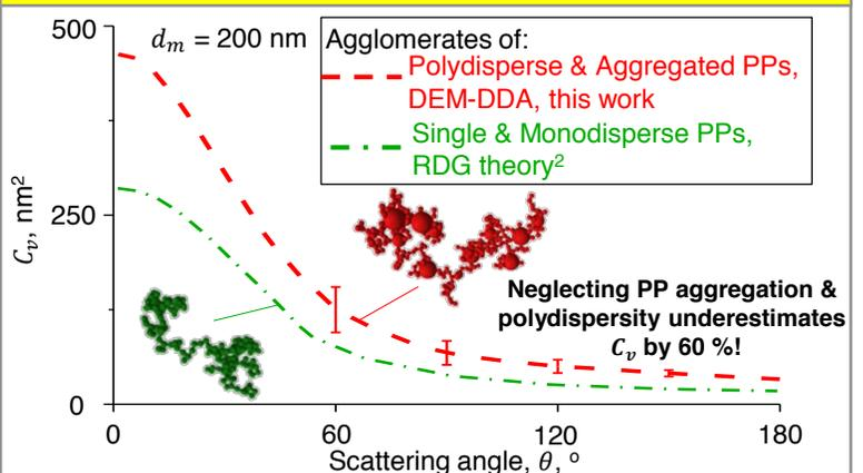
The  $C_v$  of DEM-derived soot agglomerates of polydisperse & aggregated PPs with  $d_m = 200 \text{ nm}$  estimated by DDA (broken line) compared to the RDG theory for agglomerates of single & monodisperse PPs with the same  $d_m$  (dot-dashed line).
