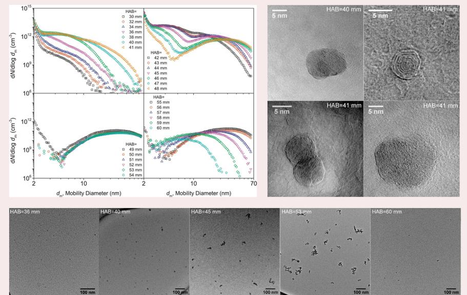
Fig. 3. Size distribution and TEM images of particles from HAB = 30 to 60 mm
