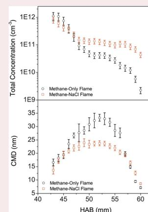
Fig. 5. Variation of count median diameter (CMD) and total number concentration of particles for HAB = 43–60 mm for methane-only and methane-NaCl flames.
