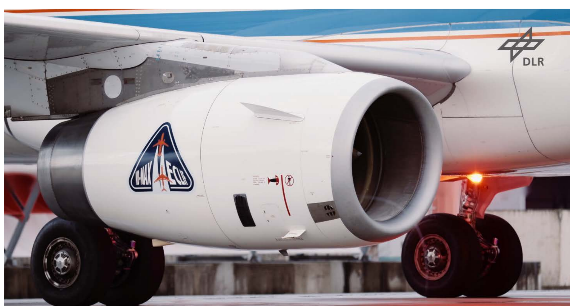
Figure 2. The V2527-A5 engine used in this study, mounted on the DLR ATRA A320 aircraft.
