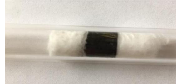
Plug flow reactor with packed bed
