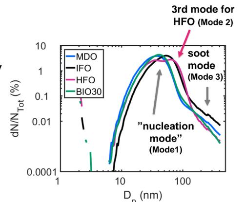
Figure 3. Normalised particle number size distributions at 25% load.
