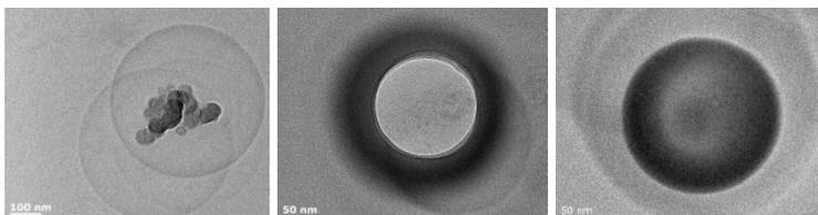
Beam contamination in form of characteristic dark rings. Arises due to degradation of oil adsorbed onto surface of soot nanoparticles that have been extracted from lubricant oil phase of a GDI engine.
