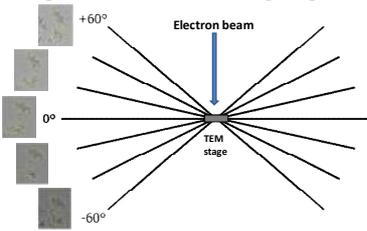
**Reconstruction Algorithm:** Single-axis weighted back-projection (WBP), Dual-axis WBP, Simultaneous Iterative Reconstruction Technique (SIRT)
