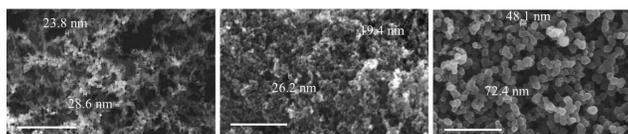
**Figure 3.** SEM images of soot from the three flames shown in Figure 2. Recirculation increases  $d_p$  for soot particles. Scale bars represent 500 nm.
