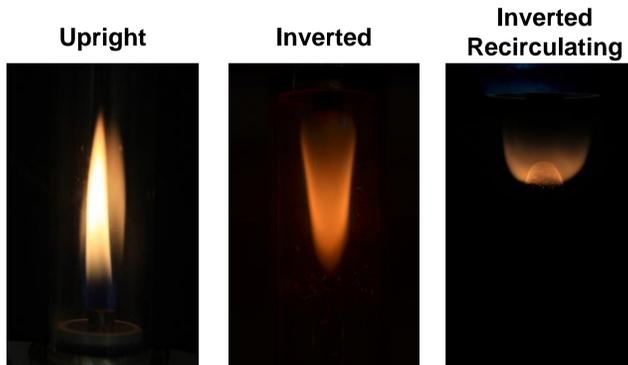
**Figure 2.** Three methane diffusion flames studied. Soot at the base of the recirculating flame is observed flowing from the flame front back inside of the high temperature fuel rich region.
