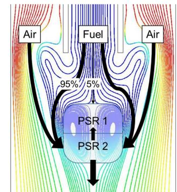
**Figure 7.** CRN created from experimental observations and CFD simulations. The PSR is composed of three main components, a PSR modeling the fuel rich region conducive to primary particle growth, a second PSR at stoichiometric conditions that carbonizes and solidifies soot particles, and a recirculation region that carries soot from the flame front back inside of the fuel rich region.
