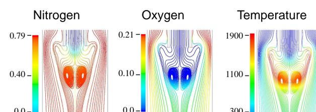
**Figure 5.** Pathlines of the gaseous flow inside the IGFR recirculating flame. Left: Nitrogen mole fraction profile. Middle: Oxygen mole fraction profile. Right: Temperature profile. Temperature includes heat radiation from soot production. Peak flame temperature is 1920 K.
