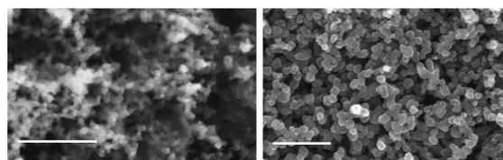
**Figure 4.** Ethylene diffusion flame soot. A recirculating flame creates fractals with a consistently larger  $d_p$ . Left: SEM image of soot produced in upright ethylene flame with  $d_p$  in typically reported range. Right: SEM image of soot produced in ethylene IGFR recirculating flame.
