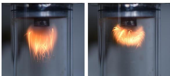
**Figure 1.** Hydrogen diffusion flames with tracer particles injected to visualize pathlines (streaks). Left: High fuel inlet with no recirculation. Right: Flow moves axially from the nozzle until convective and buoyant forces drive the particles to recirculate and move upwards towards the fuel inlet.
