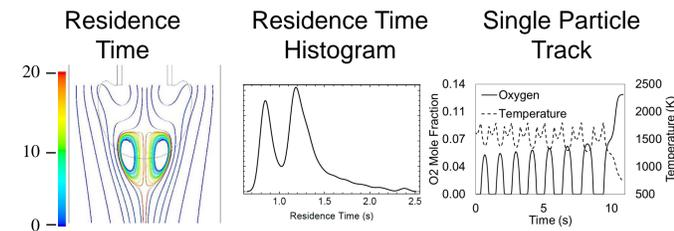
**Figure 6.** Left: CFD showing recirculating pathlines and resulting residence time. Particles in the entrainment have residence times up to 20 seconds. Middle: Probability distribution of residence times. Right: The surrounding oxygen and temperature of a single particle entrained for 10 seconds inside the recirculation region. The particle oscillates between rich and lean regions of the reactor.
