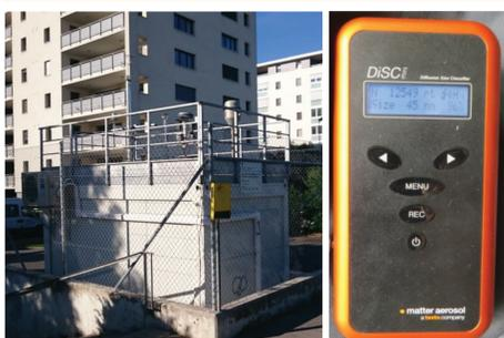
Fig. 6 Analysis of ambient air. Left: the official analysis station of the city of Fribourg (Perolles). Right: DiSC-mini of Testo.
