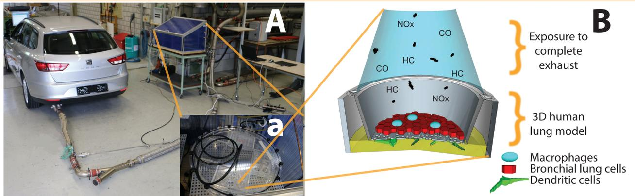
Fig. 1 Exposure setup. [A] An exposure box (blue) is directly connected to the exhaustpipe of a passenger car. The exposure box contains two chambers ([a] filtered air and exhaust). [B] Scheme of the human lung model composed of three different human cells. The cells are at the air-liquid interface, air (or exhaust) on top, and medium on the bottom [3].
