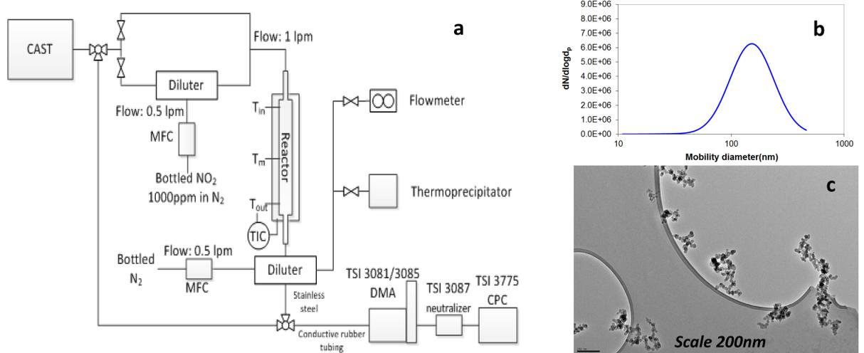
Figure 1: a- Schematic diagram of the experimental setup, b- mobility particle size distribution of the CAST-generated soot, c- TEM image of CAST-generated soot particles
