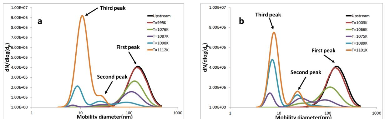
Figure 2: The particle size distribution (PSD) of CAST-generated aggregates for different T using a) oxA, and b) oxB.
