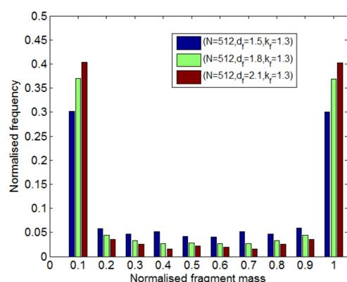
Figure 5: The normalized frequency of the aggregates mass fraction after a single-neck breakage, divided in 10 bins.
