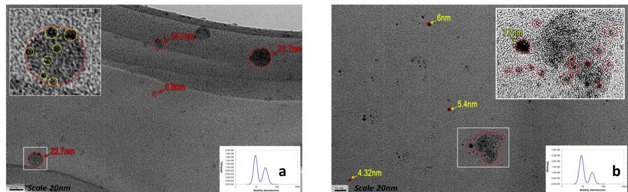
Figure 4: TEM images and the corresponding PSD for a) oxA, and b) oxB(right).
