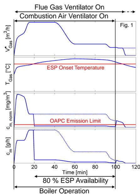
**ESP Operating Points:** Due to the lack of a reliable and affordable sensor to continuously measure PM emissions from biomass combustion, ESP operation has to be monitored depending on applied voltage and current.
