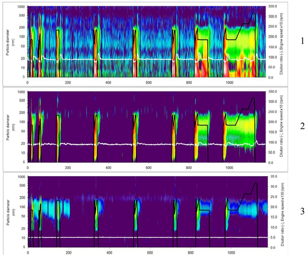
**Figure 3: DMS500 spectra for 3WC upstream (1), 3WC downstream (2) and GPF downstream (3) positions for a conventional vehicle**
