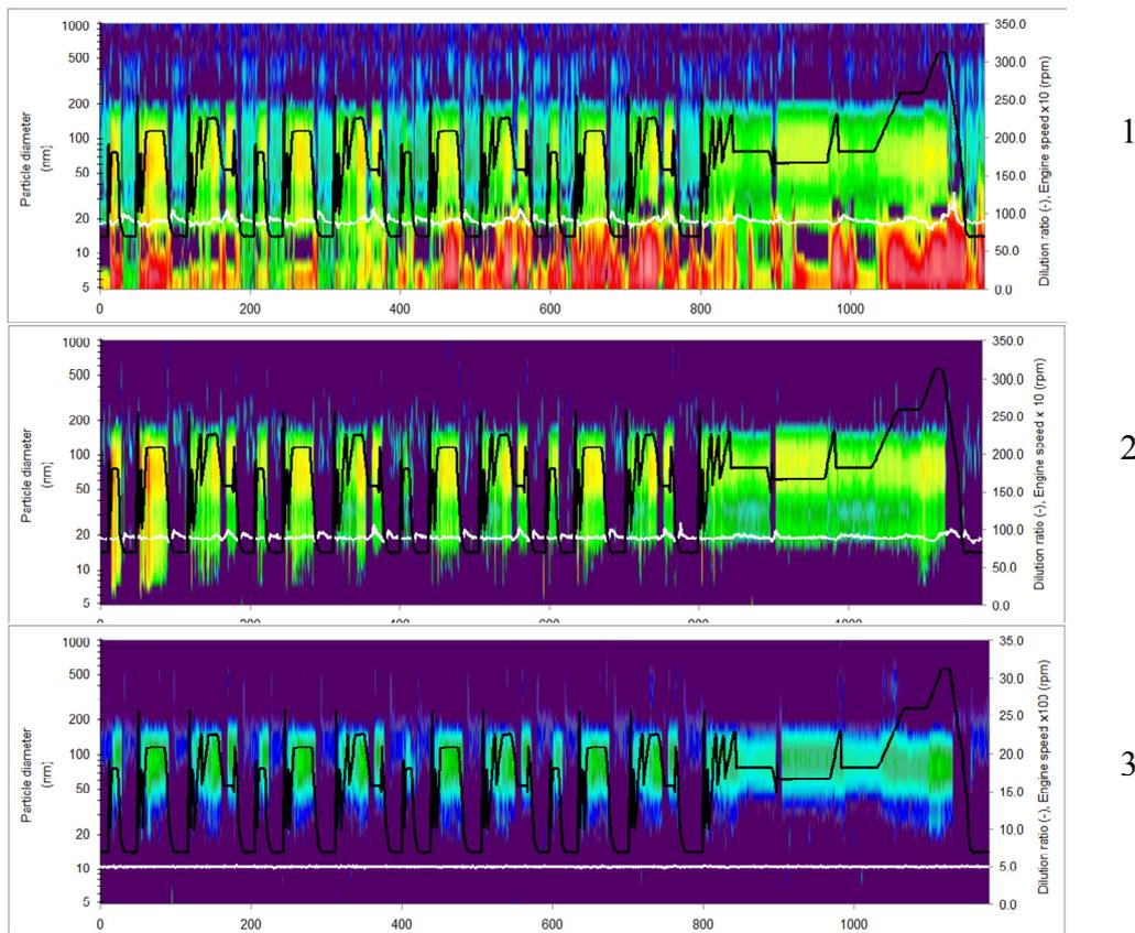
**Figure 2 : DMS500 spectra for 3WC upstream (1), 3WC downstream (2) and GPF downstream (3) positions for a conventional vehicle**
