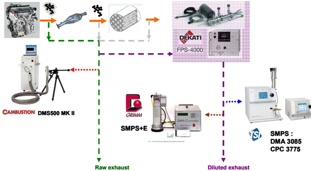
**Figure 1 : Experimental setup for the GDI engine particles characterisation with DMS500, SMPS TSI and SMPS+E Grimm**
