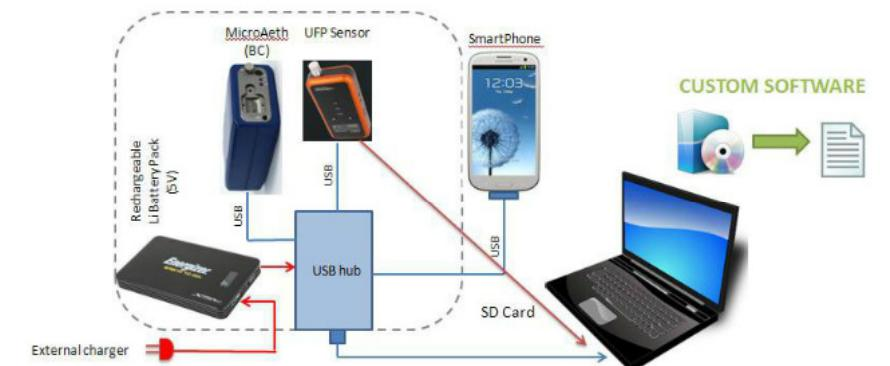
Figure 4 - Data extraction and battery recharge (KOM concept)
