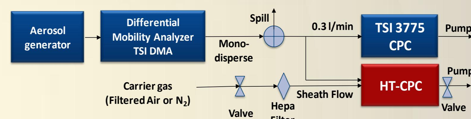
The HT-CPC and TSI CPC were compared and the counting efficiency as a function of particle electrical mobility diameter was obtained.
