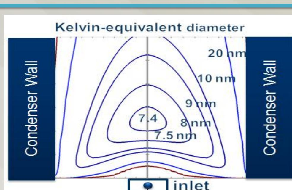
The model suggested that the HT-CPC will be able to grow and detect solid nanoparticles and remove tetracontane volatile particles at the same time. A prototype was then designed and built based on the model simulations.
