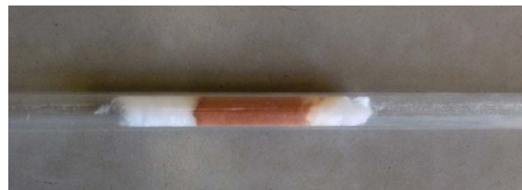
Plug flow reactor with packed bed
