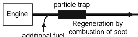
Figure 5: Schematic diagram of a particle trap
