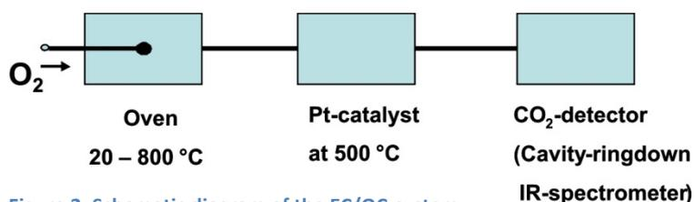
Figure 2: Schematic diagram of the EC/OC-system
