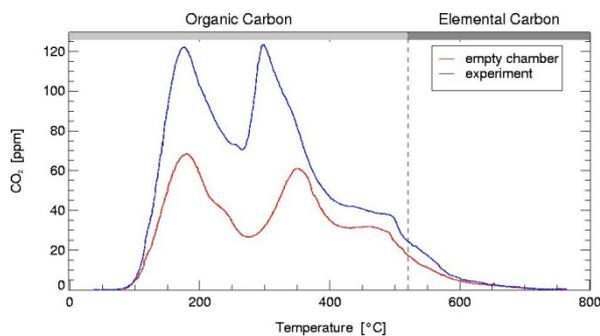
Figure 7: The OC-fraction shows a significant rise between the empty garage (red) and the experiment (blue).
