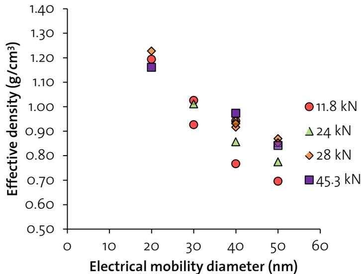
Figure 3. Effective density as a function of particle size and engine thrust.
