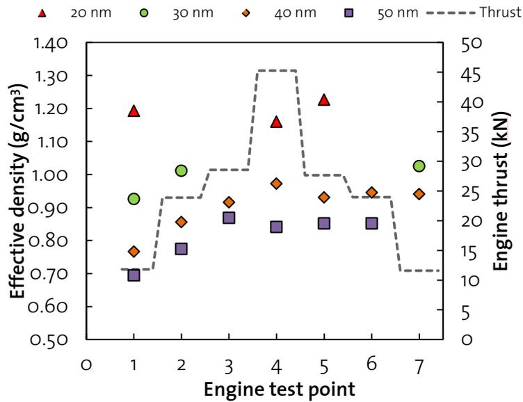
Figure 2. Size-resolved effective density obtained per engine test point. Test point duration was 16 minutes.
