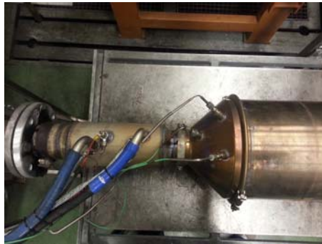
Regeneration burner and DPF (right)
