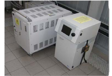
Equipment for quantification and characterization of particulate matter emissions – filter holder installation, particle counter, particle sizer
