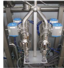
Equipment for quantification and characterization of particulate matter emissions – filter holder installation, particle counter, particle sizer
