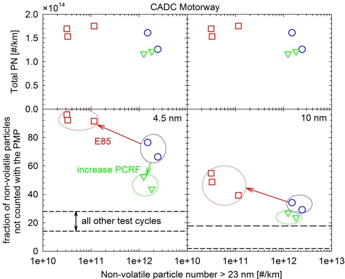
⇒ Excessive particle counts downstream of the VPR under conditions favouring nucleation mode formation in the CVS tunnel
