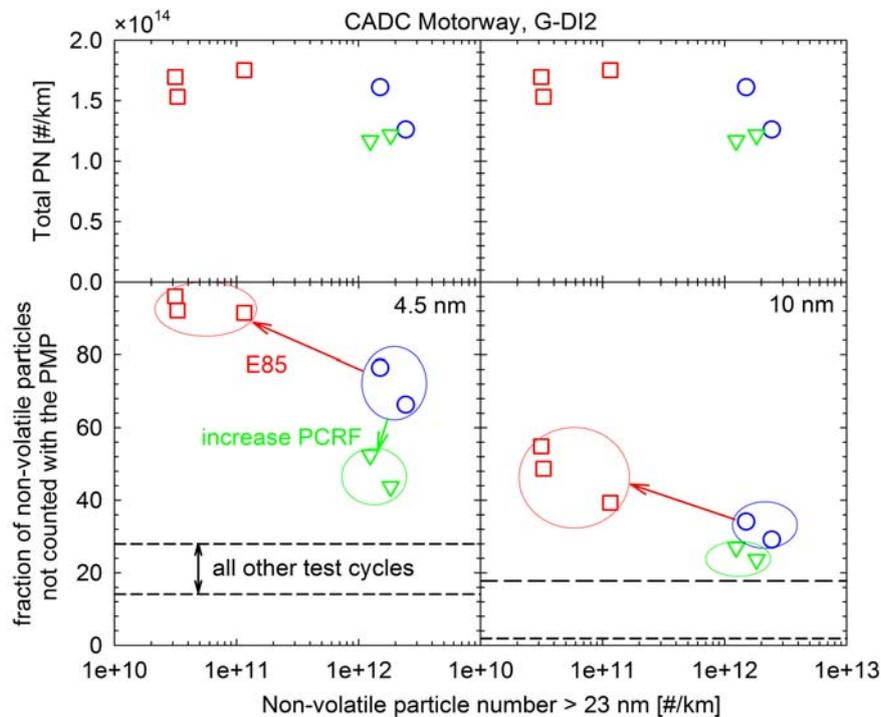
Figure 2: Dependence of the fraction of excess particles detected by CPC@4.5 (left-hand panel) and CPC@10 (right-hand panel), on the dilution ratio (3500:1 for green symbols, 2000:1 for blue and red symbols) for a flexi-fuel G-DI tested on 5% ethanol (blue-green symbols) and 85% ethanol (red symbols).
