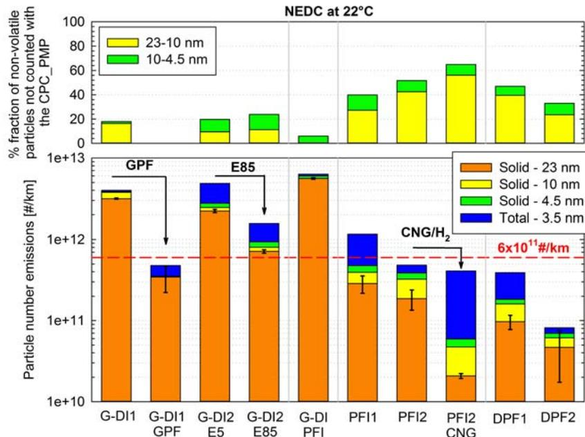
Figure 1: Lower panel: Overview of the particle number emissions over the NEDC, determined with the different CPCs. Upper panel: fraction of non-volatile particles not detected by the CPC@23.
