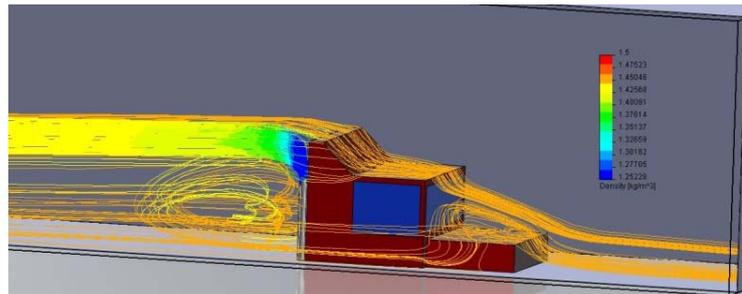
Figure 2: CFD Simulations, Exhaust stack lower than fairing
