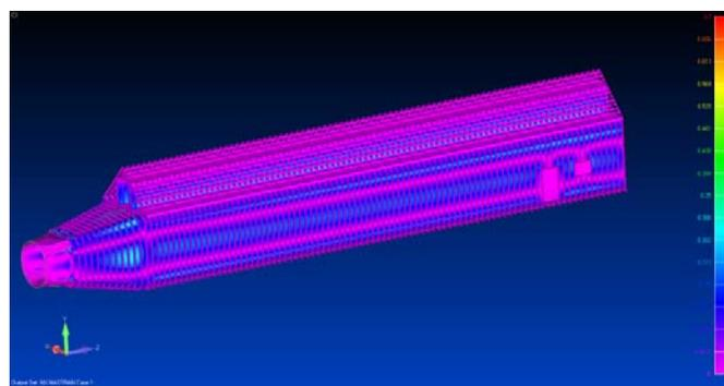
Figure 3: FEA results for operational conditions (load set 1), failure index contour plot
