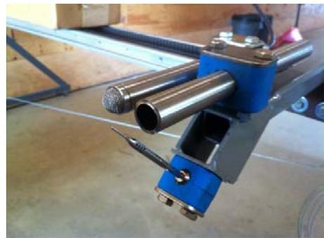
**Figure 4: Exhaust plume sampling probe and flow field characterization sensors**
