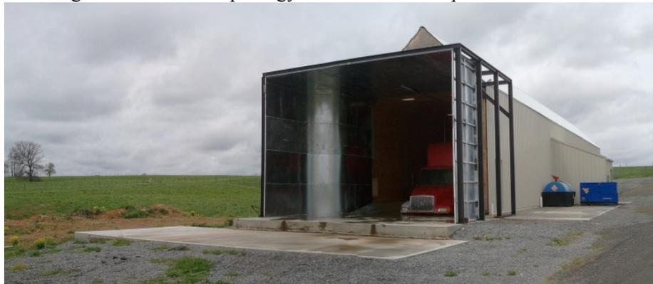
**Figure 1: WVU wind tunnel with mock up truck visible inside**
