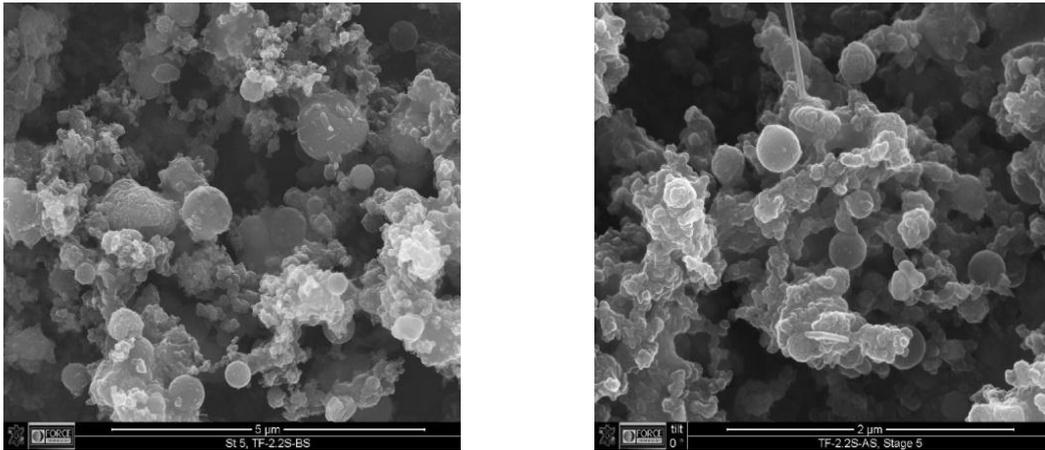
**Figure 4:** Representative SEM images of particles collected on ELPI stage 5 (260-380 nm) before and after the scrubber using 2.3 % S fuel. Note the different scaling
