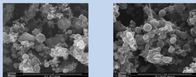
Figure 4: Representative SEM images of particles collected on ELPI stage 5 (260-380 nm) before and after the scrubber using 2.3 % S fuel. Note the different scaling
