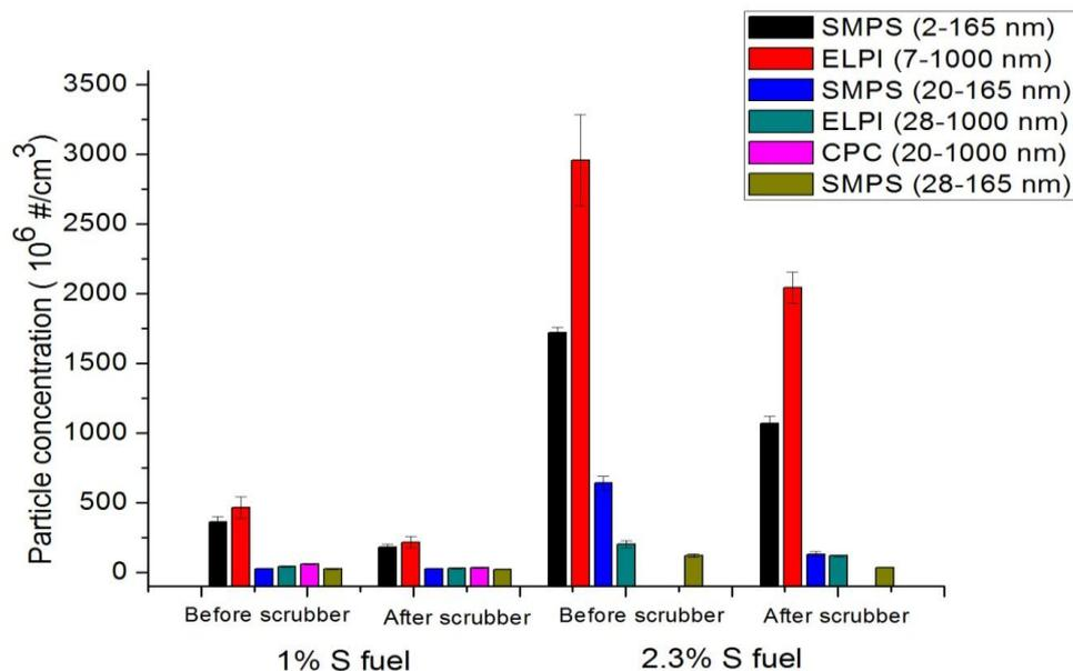
**Figure 3:** Comparison of PN concentration measured by SMPS, ELPI and CPC for 2.3 % S fuel and 1.0 % S fuel. (SMPS: mobility diameter, ELPI: aerodynamic diameter)
