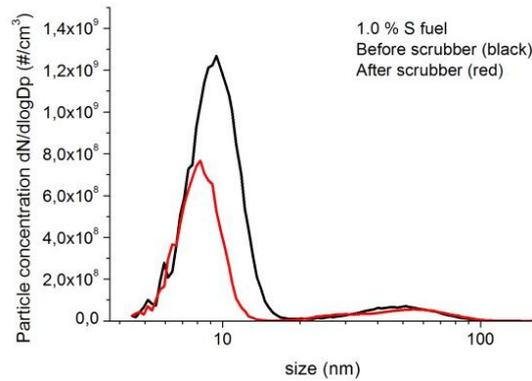
**Figure 2:** Particle size distributions measured by SMPS before and after the scrubber using 1.0 % S fuel.
