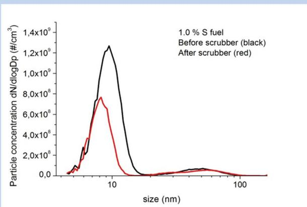
Figure 2: Particle size distributions measured by SMPS before and after the scrubber using 1.0 % S fuel.
