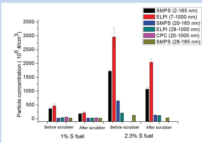
Figure 3: Comparison of PN concentration measured by SMPS, ELPI and CPC for 2.3 % S fuel and 1.0 % S fuel. (SMPS: mobility diameter, ELPI: aerodynamic diameter)
