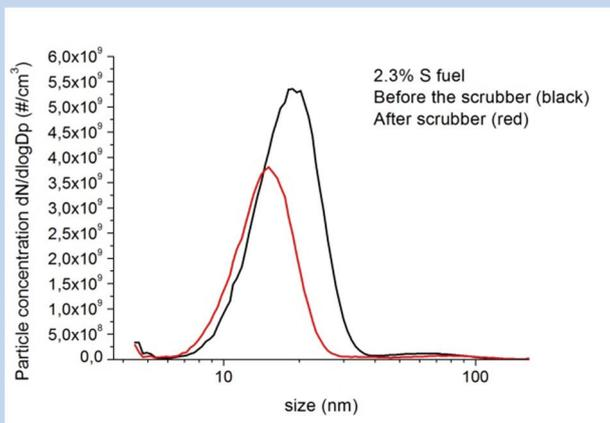
Figure 1: Particle size distributions measured by SMPS before and after the scrubber using 2.3 % S fuel.
