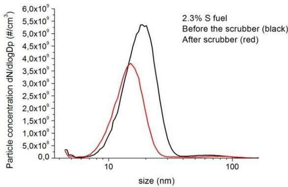
**Figure 1:** Particle size distributions measured by SMPS before and after the scrubber using 2.3 % S fuel.
