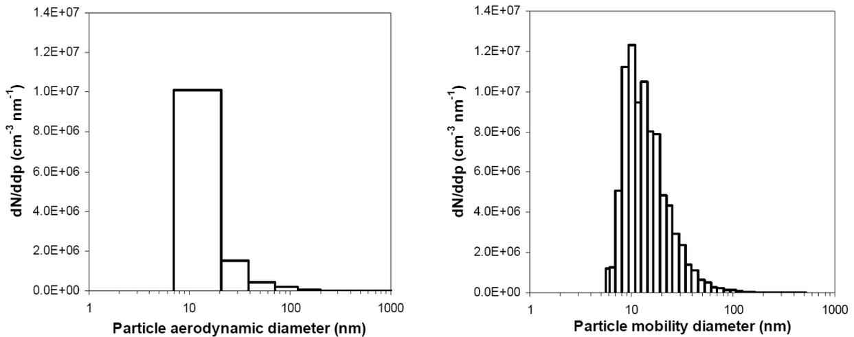
Figure 5. Average size distribution given by ELPI (left) and FMPS (right)
