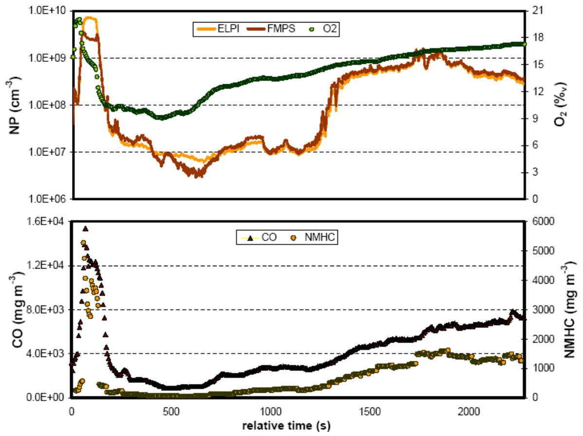
Figure 3. Time profiles for a) NP number measurements and flue gas oxygen content, b) CO and NMHC concentrations
