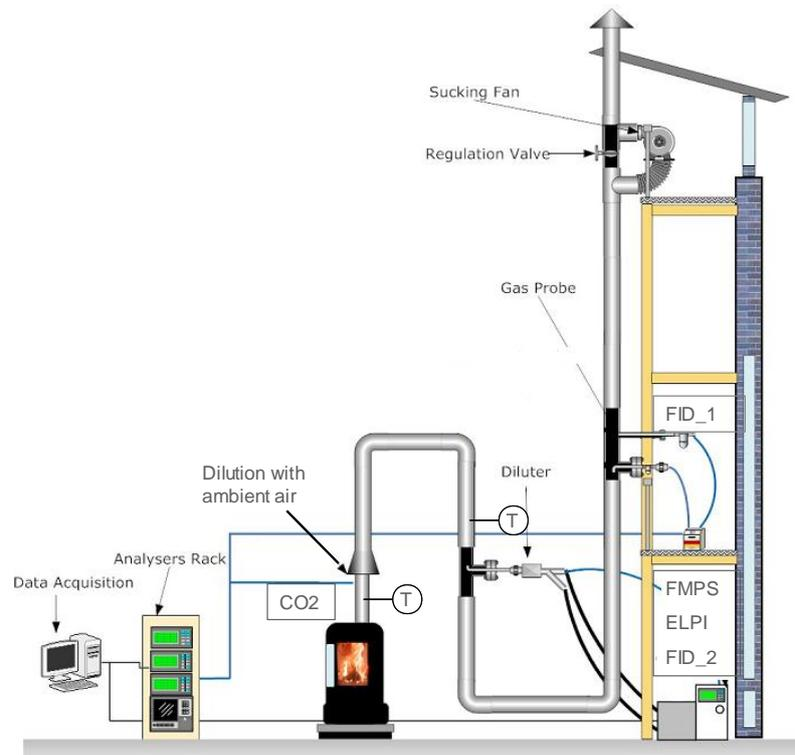
Figure 1. Schematic of the experimental test rig
