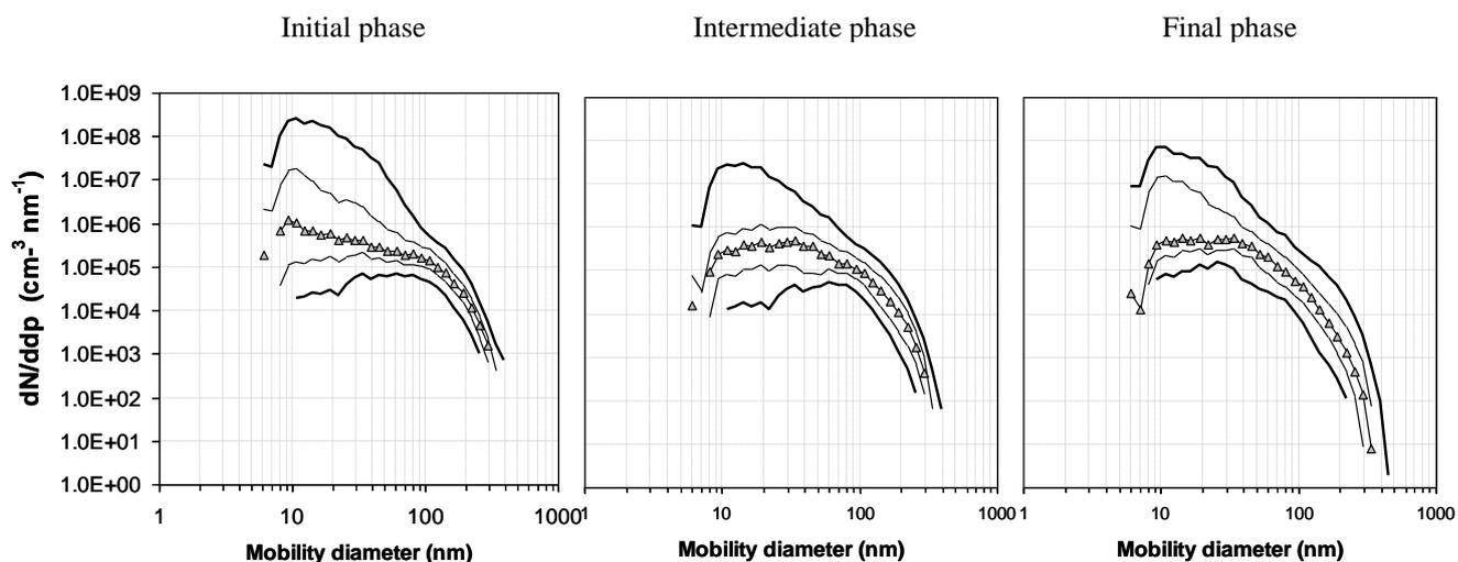
Figure 7. Phase resolved size distributions of particles (5<sup>th</sup>, 25<sup>th</sup>, 50<sup>th</sup>, 75<sup>th</sup>, 95<sup>th</sup> percentiles)
