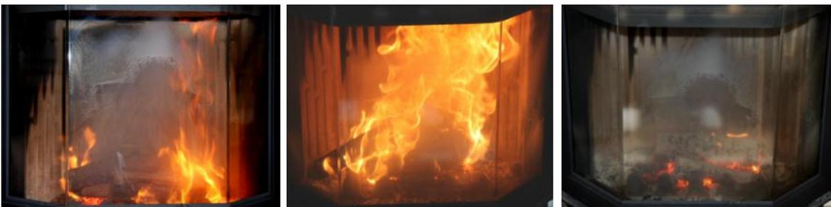
Figure 2. Visual images of the three combustion phases
