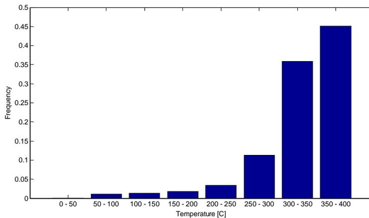
**Figure 4: Normalized exhaust gas temperature histogram for DPF inlet location, data from entire route between Morgantown, WV and Riverside, CA**
