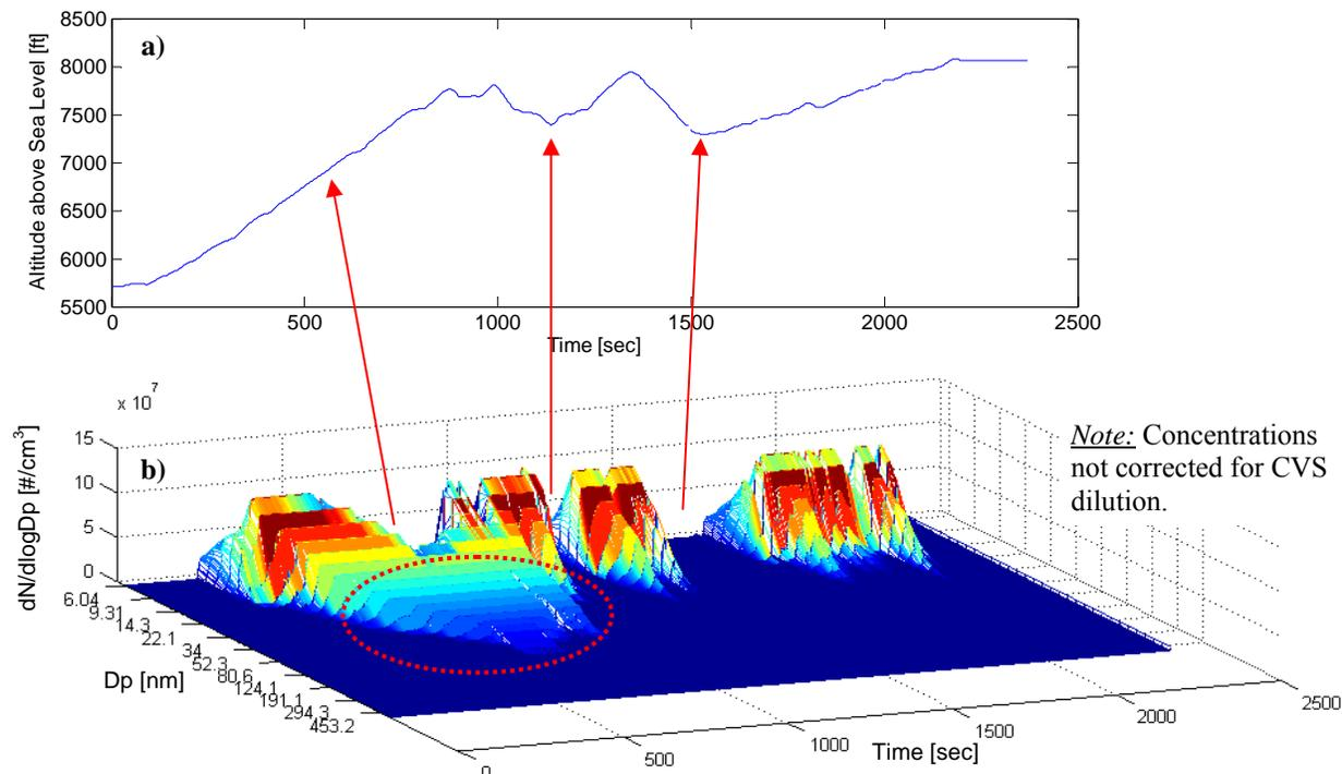
**Figure 3: a) Elevation profile for 30min highway section after Denver, CO climbing I-70 into Rocky Mountains (see), b) corresponding particle number and size distribution as measured by EEPS™, data not corrected for CVS dilution, red circle indicating DPF regeneration event.**
