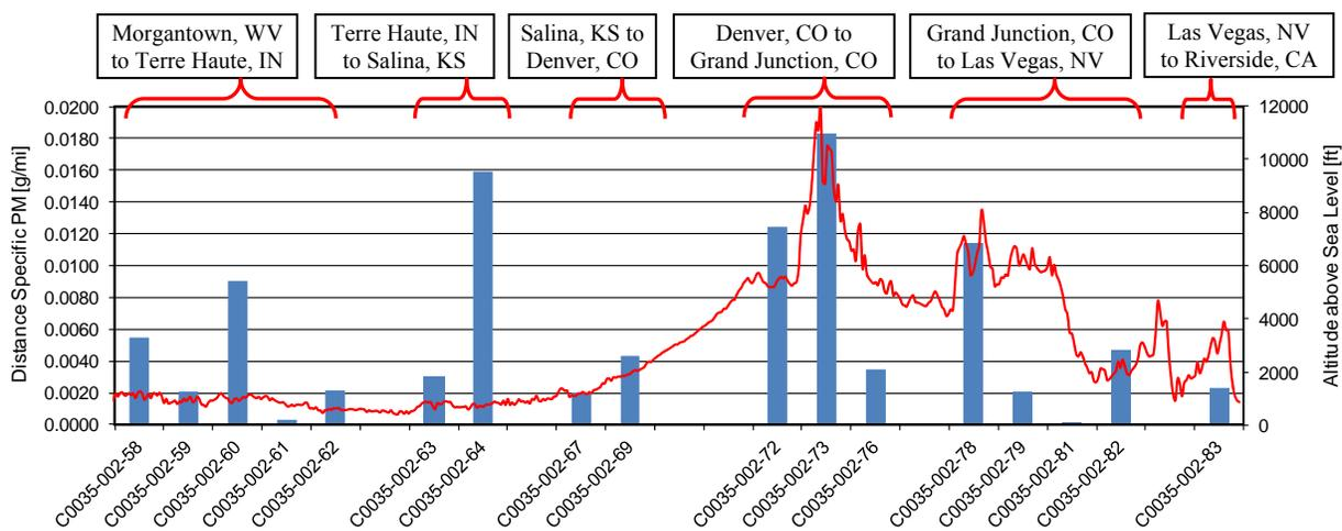
**Figure 5: Distance specific gravimetric PM emissions in [g/mi] for different portions of the route**
