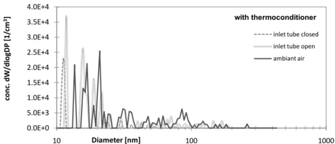
**Fig. 5:** CVS Background: Lab air and CVS tunnel only
