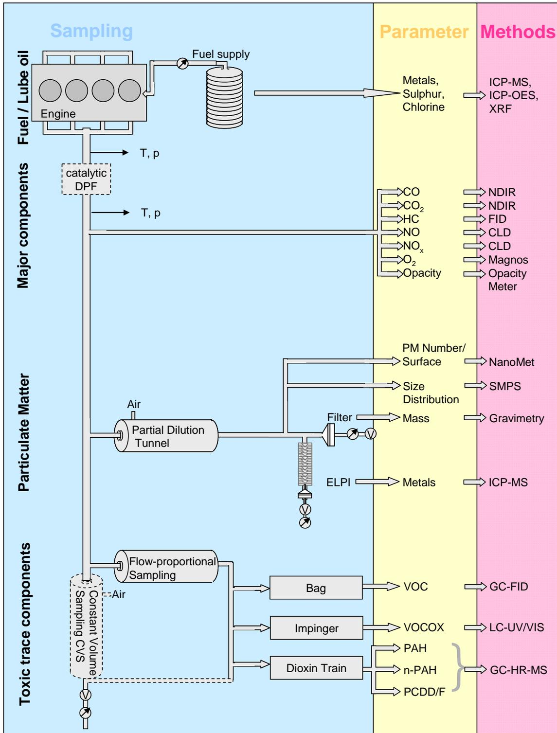
**Fig. 3:** Test and sampling setup
