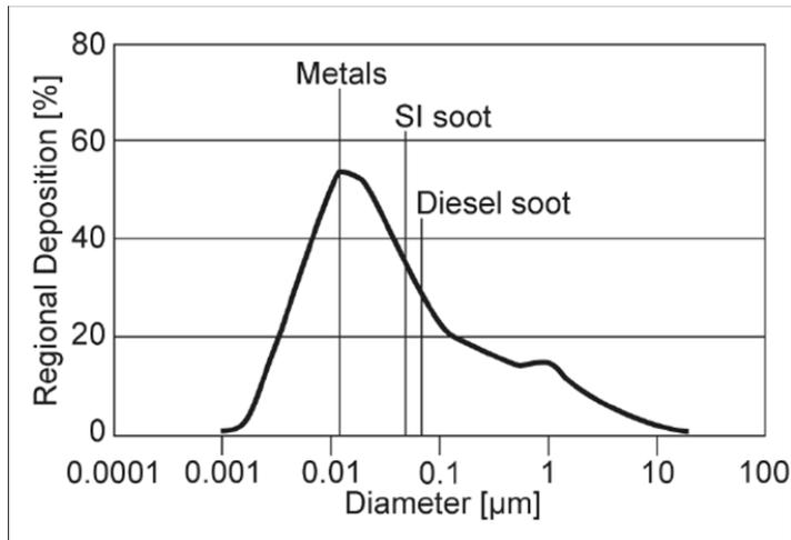
**Fig. 1:** Deposition of inhaled particles in the alveoli <sup>14</sup> The mean particle sizes are: Diesel soot about 100 nm; SI soot about 50 nm and metal oxides about 15 nm.
