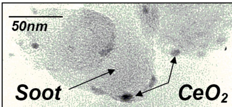
**Fig. 7:** SEM image of metal NPs, here cerium oxide, bound to soot particles
