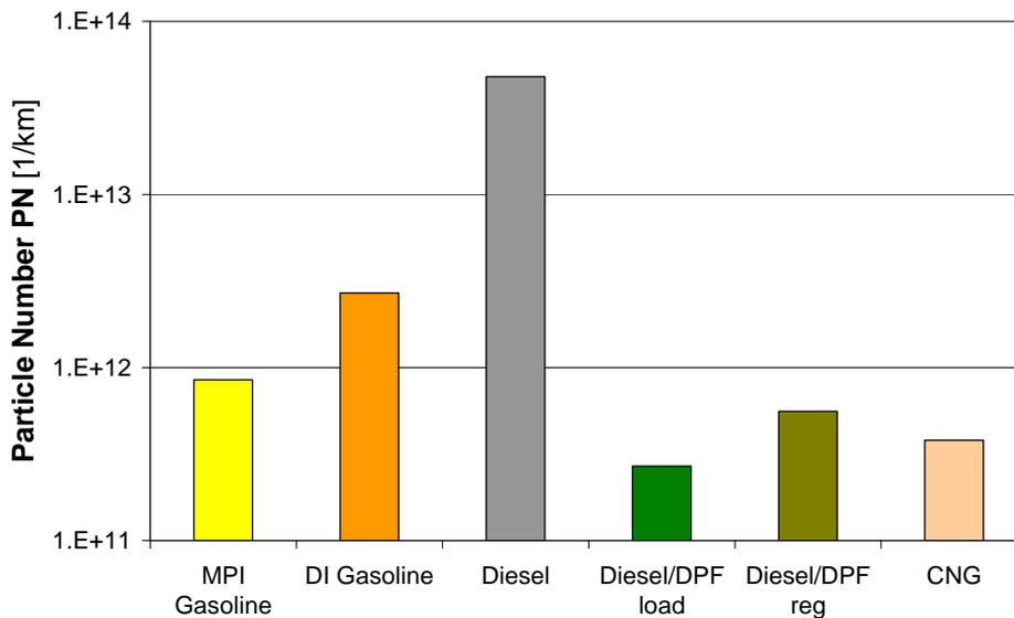
**Fig. 2:** Particle number concentration (PN) for different vehicle types
