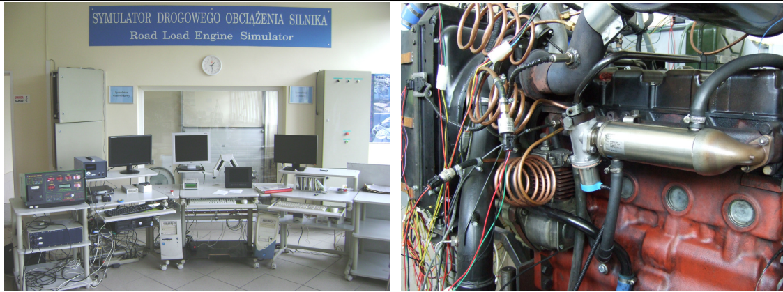
Fig. 2 Test bench Load Engine Simulator and research engine with prototype EGR valve and NO x /O 2 sensor as feedback signal
