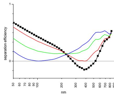
Fig. 3: Separation efficiencies. Black squares: nominal, red line: minimal agglomeration, green line: agglomeration leading to an optimally balanced separation efficiency, blue line: maximum agglomeration. The colours match those of the functions in Fig. 8.
