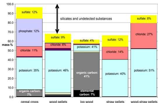
Fig. 2: Composition of dust sampled from furnaces burning different fuels. The values for calcium, nitrogen, and zinc (between organic carbon and potassium, between potassium and chloride and between chlorine and phosphorus respectively) are too small to be significant in this display. Dust was sampled on quartz filters, therefore silicates, oxides and hydroxides could not be quantified.
