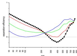
Fig. 9: Separation efficiencies. Black squares: nominal, red line: minimal agglomeration, green line: agglomeration leading to an optimally balanced separation efficiency, blue line: maximum agglomeration. The colours match those of the functions in Fig. 8.
