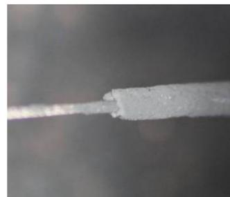
Fig. 6: Dust build-up on a charging cathode. Picture taken after only several hours of continuous operation.
