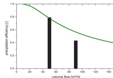
Fig. 5: Separation efficiency of a high-end electrostatic precipitator (bars) vs. its Deutsch-Anderson function. Fuel used: pure straw pellets.
