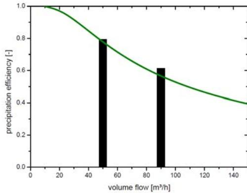
Fig. 5: Separation efficiency of a high-end electrostatic precipitator (bars) vs. its Deutsch-Anderson function. Fuel used: straw-wood composite pellets.
