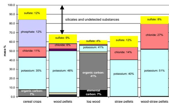
Fig. 4: Composition of dust sampled from furnaces burning different fuels. Dust was sampled on quartz filters, therefore silicates, oxides and hydroxides could not be quantified.
