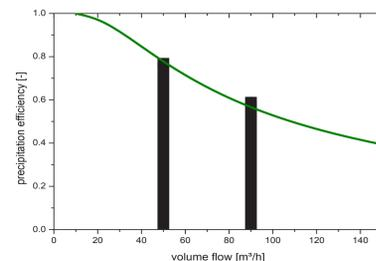
Fig. 4: Separation efficiency of a high-end electrostatic precipitator (bars) vs. its Deutsch-Anderson function. Fuel used: straw-wood composite pellets
