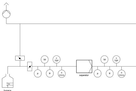
Fig. 1: Process flow diagram of the separator test bed. After the furnace the flue gas stream is divided in a part flowing through the separator and a residual stream going straight to the chimney. The flue gas is characterized by draft, flow (Prandtl's Pitot tube), temperature, gas composition and TSP (total suspended particles) are sampled.
