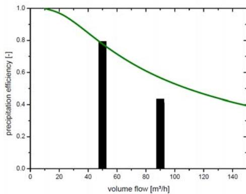
Fig. 6: Separation efficiency of a high-end electrostatic precipitator (bars) vs. its Deutsch-Anderson function. Fuel used: pure straw pellets
