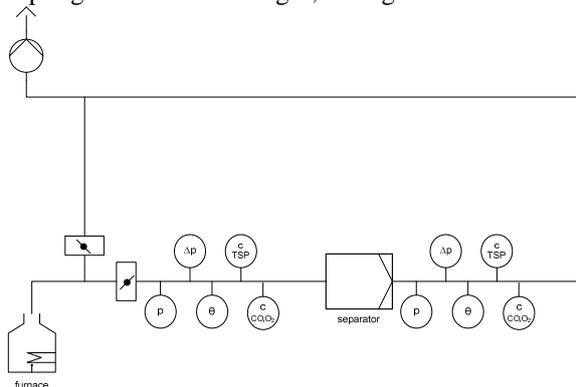
Fig. 1: Process flow diagram of the separator test bed. In order to adjust the volume flow through the separator, after the furnace the flue gas stream is divided in a part flowing through the separator and a residual stream going straight to the chimney. The flue gas is characterized by draft, flow (Prandtl's Pitot tube), temperature, gas composition and TSP (total suspended particles) are sampled.
