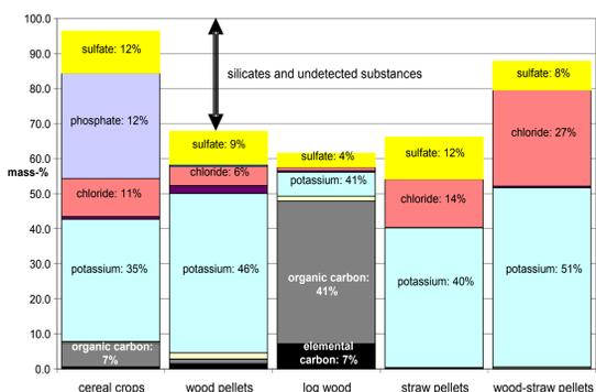
Fig. 2: Composition of dust sampled from furnaces burning different fuels. The values for calcium, nitrogen, and zinc (between organic carbon and potassium, between potassium and chloride and between chlorine and phosphorus respectively) are too small to be significant in this display. Dust was sampled on quartz filters, therefore silicates, oxides and hydroxides could not be quantified.
