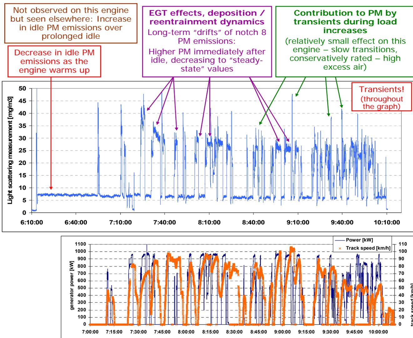
**Measurement of exhaust emissions of railroad locomotives using an on-board system**
