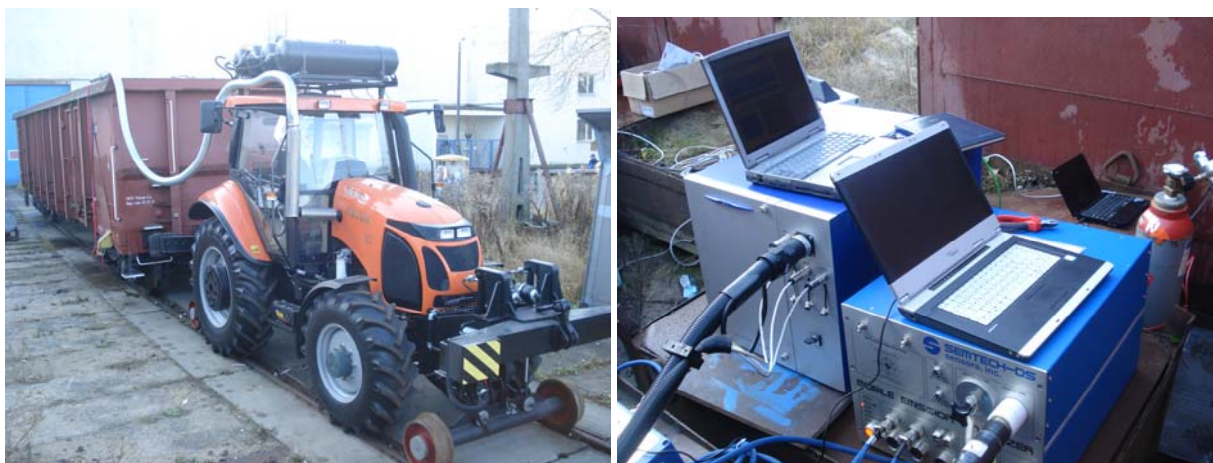
Fig. 1. The tests of Crystal tractor with fitted systems of exhaust emission measurement carried out in RVI Tabor in Poznan
