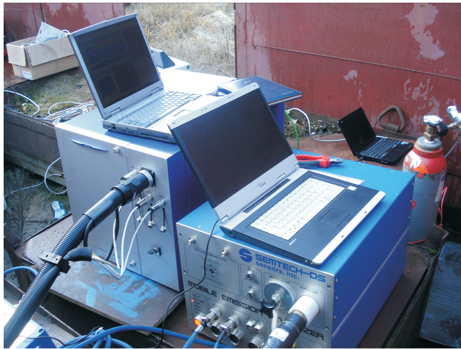
The tests of Crystal tractor with fitted systems of exhaust emission measurement
