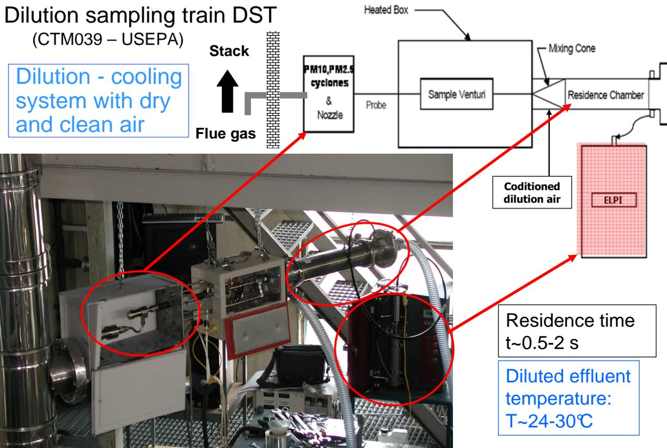
Dilution - cooling system with dry and clean air
