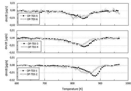
Soot samples on a quartz glass filter were dried in N<sub>2</sub>-atmosphere up to 873K prior to the temperature programmed oxidation in synthetic air.
