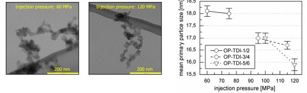
The size distribution of primary particles is determined by measuring multiple soot agglomerate images from samples of each operating point
