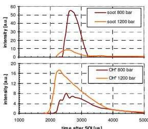
The OH\*/soot ratio rises for operating points with higher injection pressure
