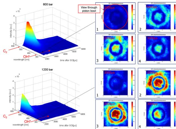
→ Ratio of integrated in-cylinder OH\* and soot (C<sub>2</sub>) chemiluminescence signal is compared
