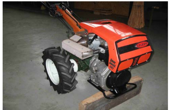
Figure 4: Rotary cultivator with retrofitted diesel particulate filter
