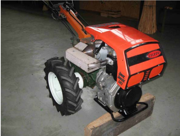
Figure 4: Rotary cultivator with retrofitted diesel particulate filter (cutter unit missing)
