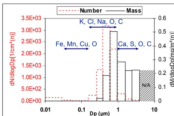
**Figure 2.** Most abundant elements found by EDX analysis of the particles emitted from the landfill gas fired CHP plant GF2.
