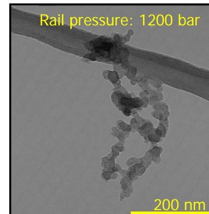
Primary particle mean size is reduced for increasing rail pressure
